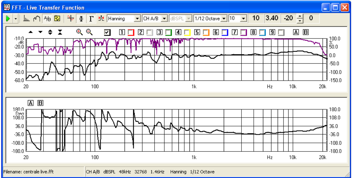
Fig. 9.3 The Live transfer function control panel
