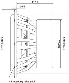
with pockets Ø9,5 equispaced on Ø256
